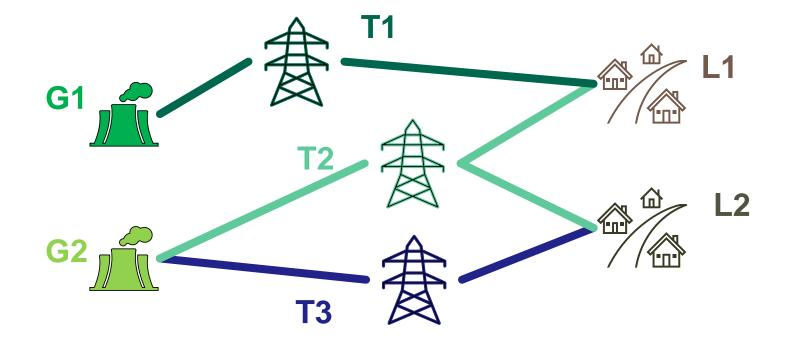
The system works if both loads are satisfied, which happens if each community is connected to at least one working generator. Suppose that there is a seismic risk for the power plants and the transmission lines and when an earthquake occurs, there is a probability that the generators and the transmission lines are disconnected. Assuming that:
