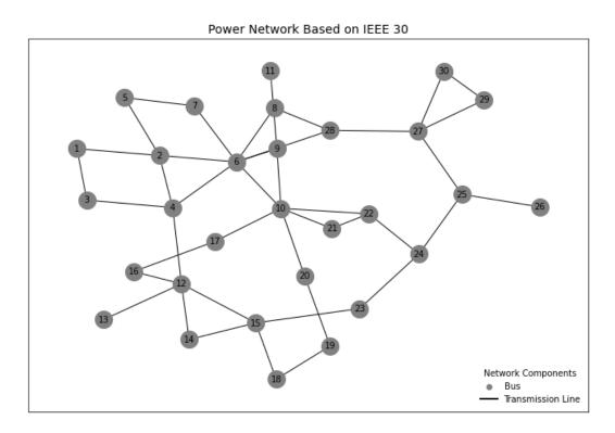
All nodes have buses that act as hubs where electrical power is either injected (from generators), withdrawn (by loads), or transferred across the network. If a bus fails, the corresponding node becomes inoperable
