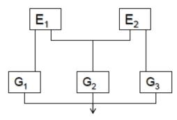
E1, E2 = engines G1, G2, G3 = generators, each one is rated at 30 KVA
